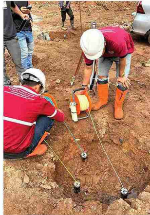
Sonic Logging Test (CSL- Test)
